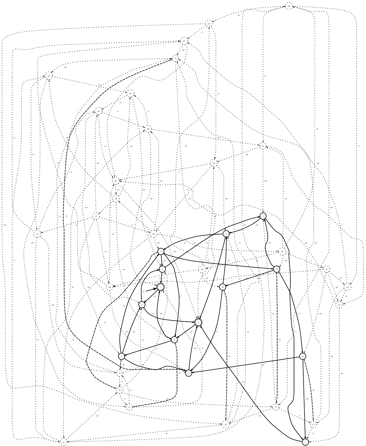
Fig. 6. Controlled process H : figure without dotted-lines; Updated controlled process H_{updated} : complete figure. The dotted and dashed lines represent the part of behavior that has been added by the updated or new behaviors and specifications. Precisely, the dashed-lines represent the event f_2 and where the updated behavior starts.
